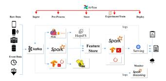
Figure 1. End-to-End ML Pipeline, orchestrated by Airflow
